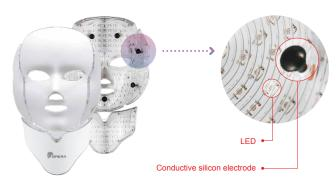
Simultaneous operation of LED and galvanic currents flowing in the galvanic electrode.
